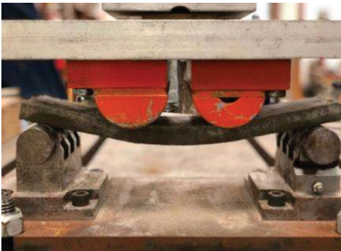
High deflection capacity of Engineered Cementitious Composites (ECC) material developed at LSU
